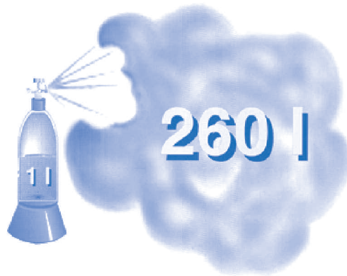
Figure 2.4. Evaporation of even small quantities of flammable liquids (such as liquefied propane) may give rise to large quantities of flammable vapours
