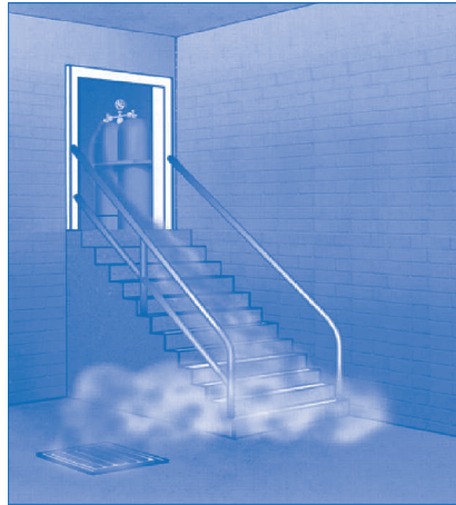
Figure 2.3. Spread of liquefied gases (example) (6)
